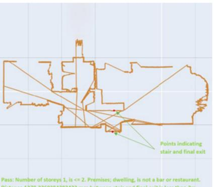
Distance 1279.3269384382422 mm between stair and final exit is less than 3m.
